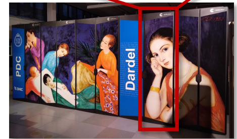
Dardel: 56 nodes, 448 MI250X GCDs, ≈10 PFlop/s
